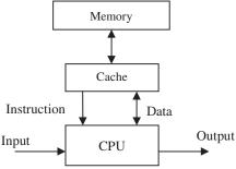
Figure 2: Modified Harvard Architecture
